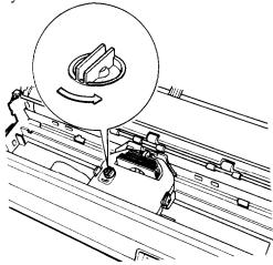
7. Holding the print head, slide the print head from side to side to make sure that it moves smoothly. (Do not try to slide the print head by grasping the ribbon cartridge.)
